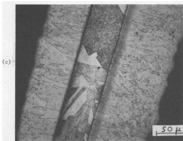
Fig. 9. Nb deposit obtained with PRC steps. i_C = 300 \text{ mA/cm}^2 ; t_C = 50 \text{ sec} ; i_A = 375 \text{ mA/cm}^2 ; t_A = 10 \text{ sec} ; Q = 4.0 . (a) Full view, (b) SEM of surface, (c) vertical cross section.
