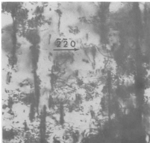
Fig. 4. A transmission electron micrograph substructure observed in a thick (Ga,Al)As layer grown on a Syton polished GaAs substrate. Plane of the micrograph is \sim(001) . Marker represents 1 \mu m.
