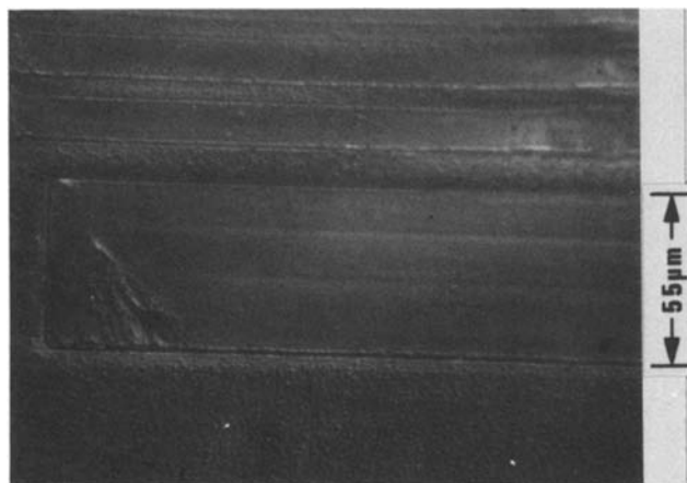
Fig. 10. An optical interference contrast micrograph of a lateral seeding sample after etching the sample in a Secco etch for 10 sec. The long polysilicon-on-oxide strip in the center of the micrograph is 194 \mu\text{m} long \times 55 \mu\text{m} wide and is completely converted to single crystal except for a small region near the corner where the beam entered the oxide substrate region. The laser scanned from left to right and the lines stepped from top to bottom.
