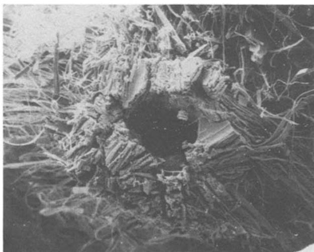
Fig. 10. Cross section of a copper wire completely reacted with \text{COCl}_2 . 100 \times .
