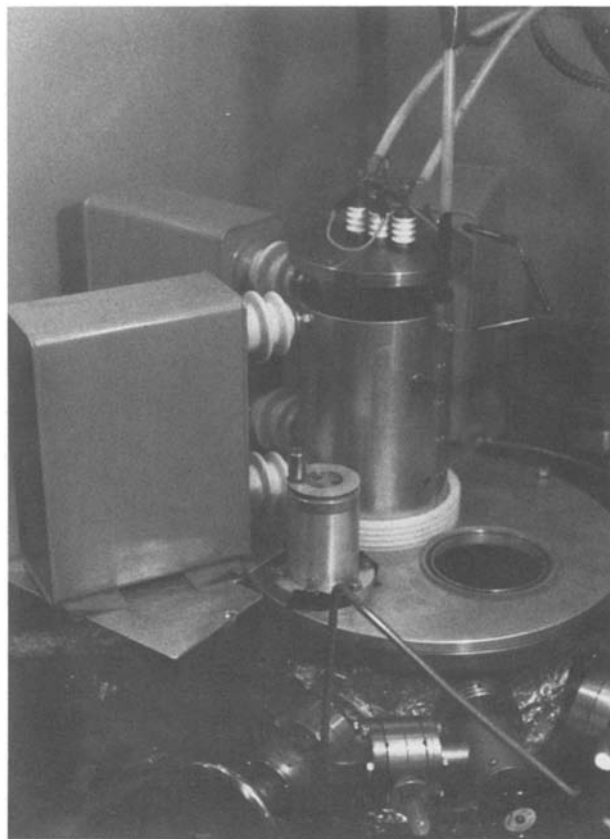
Fig. 2. Pulsed electron beam apparatus
