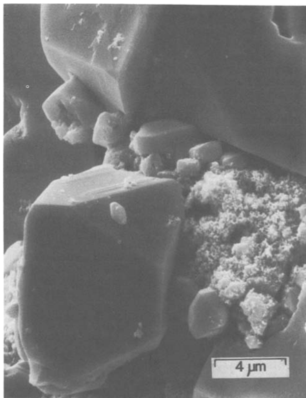
Fig. 4. Positive active material at the end of cycle 1 discharge at 18 \text{A/m}^2 , the 24 hr rate. The smallest particles are \text{PbO}_2 . Medium size and large crystals are \text{PbSO}_4 .
