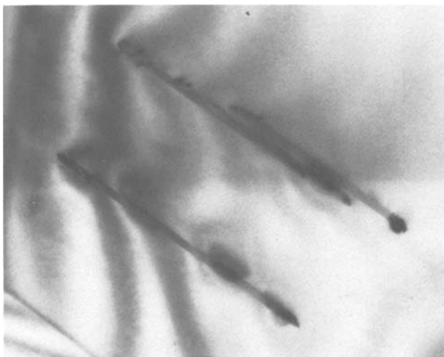
Fig. 2. TEM photo of small stacking fault formed during initial oxidation.
