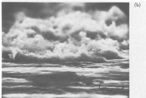
Fig. 7. Scanning electron micrographs of a stripped lithium electrode surface which has undergone three complete cycles. In (b), the sample has been tilted \sim 90^\circ with respect to the substrate in order to estimate film thickness.
