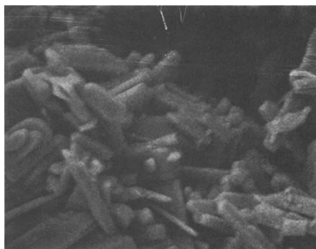
Fig. 2. SEM photograph of Fe substituted vanadium oxide. Magnification 1000 \times .
