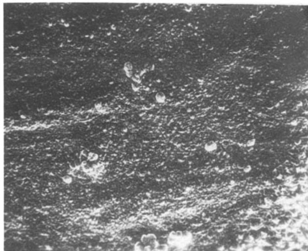
Fig. 7. Scanning electron micrographs of the Cu deposits after experiments at various cathodic d-c densities in 0.05M CuSO 4 + 0.5M H 2 SO 4 . The d-c and a-c densities (60 Hz) at which the experiments were performed are indicated on each picture. Magnification 280X.
