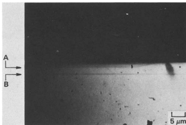
Fig. 1 Cleaved and stained cross section of a Zn diffused GaAlSb-GaSb sample. A) denotes the p-n junction location in the GaAlSb and B) denotes the GaAlSb-GaSb heterojunction interface.
