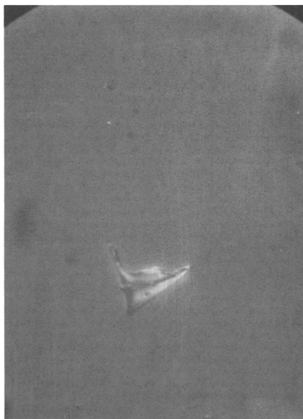
Fig. 8. Nomarski micrograph of hillock observed on the surface of a nonetched oxidized wafer. These hillocks are caused by microprecipitates present in the as-grown wafer.
