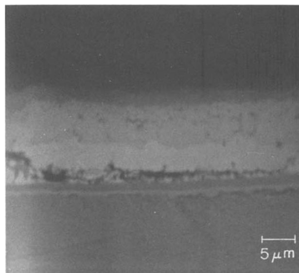
Fig. 11. An SEM cross-section photograph of Al-Au intermetallic phase. C-mode sample stored at 200°C for 10 hr demonstrates the continuous line of Kirkendall voids along the interface of intermetallic phase-gold, in "P" and "Q."
