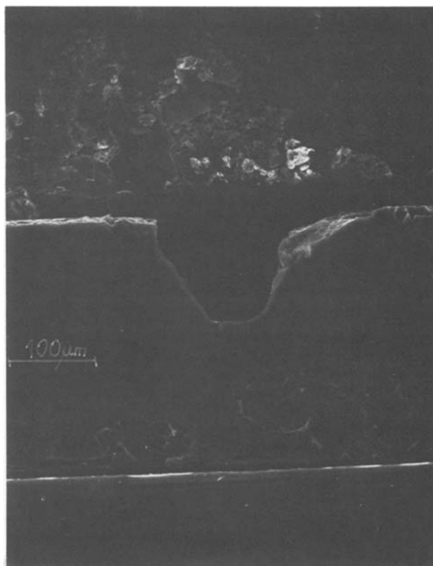
Fig. 4. Cross section of the groove after etching for 50 min, (111) wafer (SEM).
