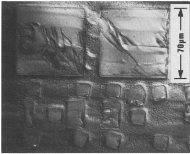
Fig. 4. An optical interference contrast micrograph of a lateral seeding area after etching in a Secco etch for 10 sec. The two large square silicon-on-oxide areas are 70 \times 70 \mu\text{m}^2 in size. The 13W laser beam scanned from left to right and the lines stepped from top to bottom.
