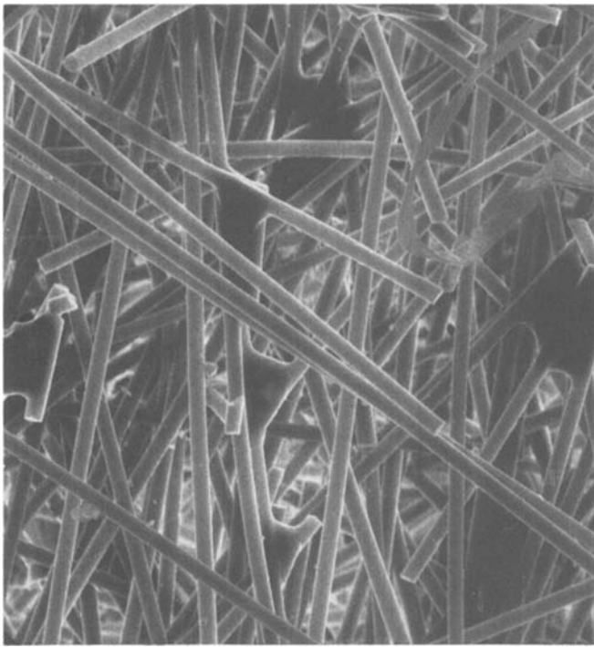
Fig. 1. Scanning micrograph of BN felt (400X)
