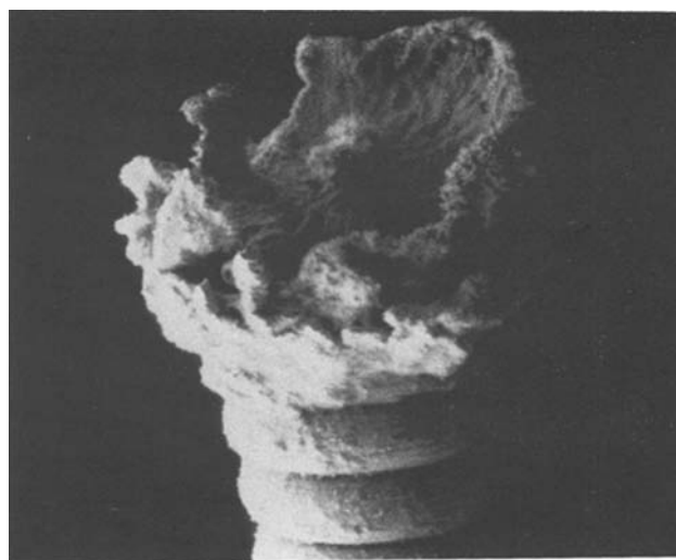
Fig. 11. Photograph of electrode originally ending in a well-defined tip after operation in discharge containing \text{ScI}_3 . This distortion also occurs in discharges containing \text{ThI}_4 .
