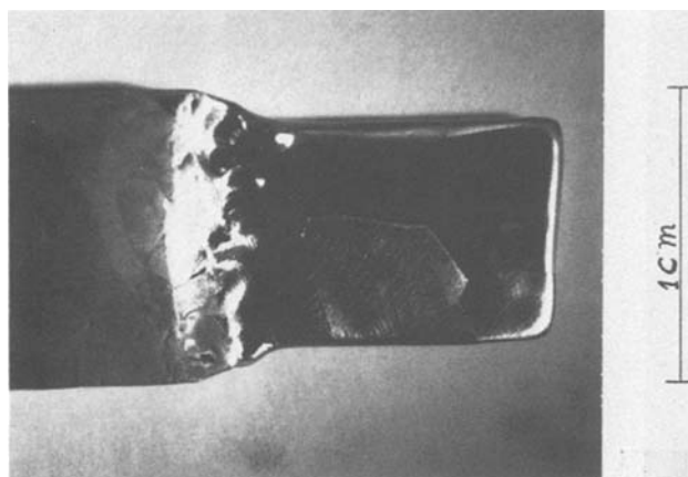
Fig. 12. Nb dissolving anode which was used in the 80 m/o K_2NbF_7 solution. i_C = 375 \text{ mA/cm}^2 ; t_C = 1 \text{ sec} ; i_A = 75 \text{ mA/cm}^2 ; t_A = 10 \text{ sec} ; Q = 0.5 .
