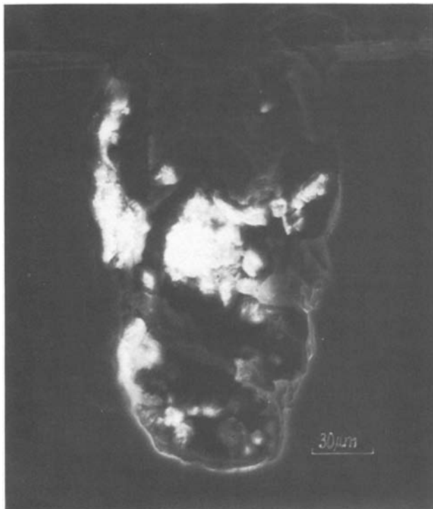
Fig. 2. Cross section through the irradiated (111) wafer. Beam parameters the same as in Fig. 1b (SEM).
