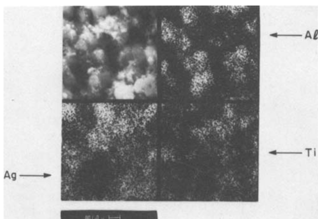
Fig. 3. SEM picture and elemental distribution maps of the TiO 2 /SIEVE paste mixture, after cell had been colored red-brown. The preferential occurrence of Ag on the TiO 2 -particles confirms their role as an in-depth contact.
