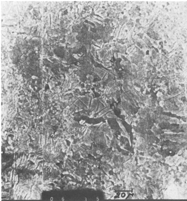
Fig. 3. SE micrograph of a magnesium electrode pretreated by standard procedure. Magnification 500X. The line drawn on the picture presents length of 20 microns.
