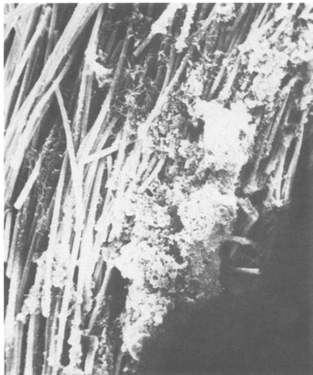
Fig. 4. SEM photograph showing boron nitride fibers, crusty reaction product, and fine fibers of the reaction product. Magnification 300 \times .
