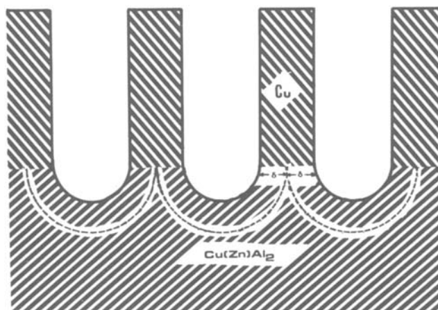
Fig. 8. Schematic representation of a Cu(Zn)Al 2 -Cu grain at the alloy-reaction product zone interface.
